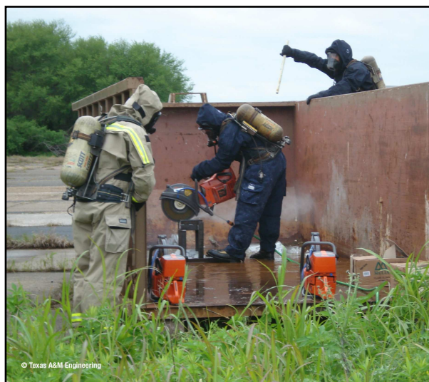
Figure 3. SMEs cut glass block as part of the multipurpose cutoff saw blade test.
