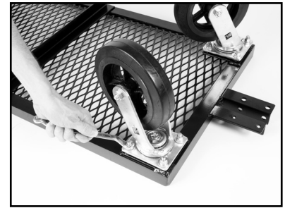
Fig. C Place swivel casters on front bolts, followed by one flat washer, one lock washer and a nut. Tighten each nut to secure caster
