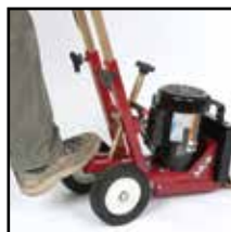
Kick plate for pivoting ease and a push-point for added force
