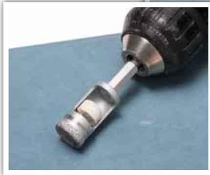
**3.** Ejector slot helps to clear the plug.
