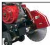
Blade guard mounts on either left- or right-hand side of saw and cuts within 2" of wall or curb
