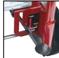
Pedal raises grinding discs off the ground for engine starting and idling.
