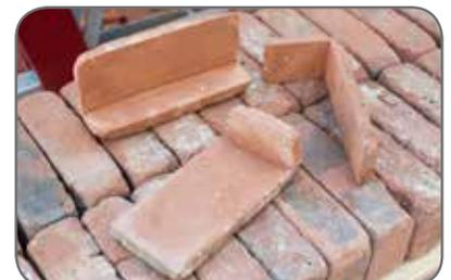
Cuts 2 x 8 right angle corners, paver corners and lintel corner.
