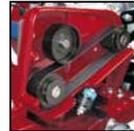
Jack shaft system on gas powered saws utilizes Micro-V belts and precision machined pulleys
