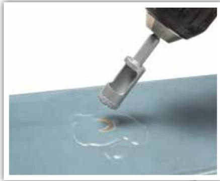
**1.** Place the raised sintered edge of the bit at a 45 degree angle to the tile. Start drilling to create a half circle.
