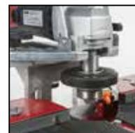
Convenient access to arbor shaft for shaping tool changes
