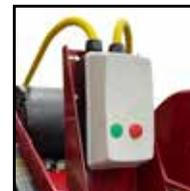
NEMA 4X rated 3PH Motor Starter is proof against rain and hose directed water. Magnetic disconnect prevents accidental restart if electrical current is disrupted.
