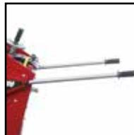
Three position adjustable solid steel handle bars
