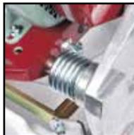
Recoil spring counterbalanced cutting head
