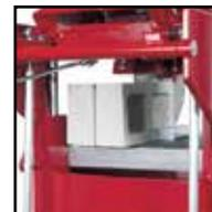
Open-back design allow for materials up to 20" long to be cut
