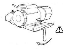
For proper operation, drive belt must be properly adjusted and in good condition. Replace the belt if worn, cracked or frayed. To adjust the belt, loosen the motor mounting nuts and adjust the motor strap tension. After adjusting the belt, be sure to retighten the motor mounting nuts.
