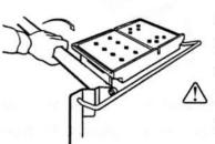
The conveyor cart may be secured into position for transportation and storage. Rotate the linear bearing guide bar cover in a clockwise direction until the conveyor cart is tight. To release, rotate the conveyor table in a counter clockwise direction until the cart moves freely.
