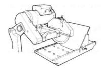
45° miter cutting is the term used to describe cutting the end of the material to a 45° bevel. Position the material against the 45° miter plate with the edge to be cut resting on the conveyor cart. Hold the material firmly against the miter plate and push the material completely through the blade.
