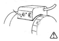
The thermal overload reset switch is located on the motor terminal cover and trips when the motor overheats. If the motor overheats, the thermal protection will cause the motor to shut off. If this should occur, allow approximately 10 minutes for the motor to cool down, then push the switch to reset.
