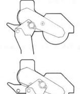
The cutting head is installed on the pivot shaft using one of two sets of holes selected by the saw operator depending on the material to be cut. The pivot hole closest to the blade is used to cut material up to 12" in size. The hole farthest from the blade is used for materials up to 16" in size.
