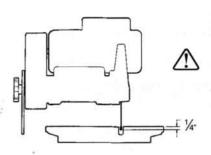
When cutting through material, the blade should penetrate at least 1/4" (6.35mm) below the surface of the conveyor cart. This adjustment is made by loosening the adjustment knob and raising or lowering the cutting head.
