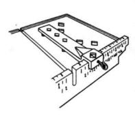
The markings on the conveyor cart backstop are used for precision cutting to exact dimensions. The scale on the top of the backstop is used for setting the rip guide alignment indicator to the desired dimension. The scale on the front face of the backstop is used to indicate the actual position of the material being cut. This offset takes into account the width between the rip guide indicator and the rip guide edge surface.
