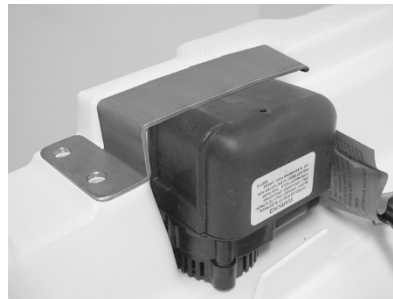
(B) Place Water Pump Clamp as shown
