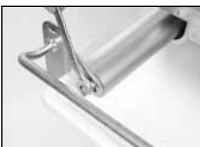
(B) Tighten Guide Bar Retaining Bolts.
