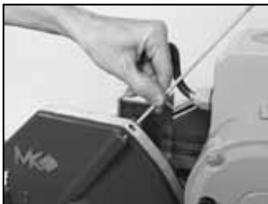
(G) Rod the Cooling Channels and then recheck flow.
