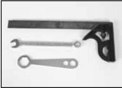
(A) Combination square (square) 12-inch or greater. 1/2-inch Wrench or MK Triple Hole Box Wrench and MK Open End Wrench.
