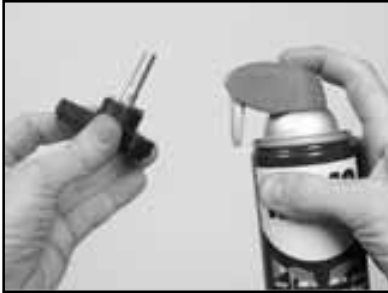
(J) Lubricate the Cutting Head Adjustment Knob.
