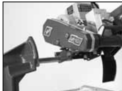
(C) Remove the Cutting Head (See Adjusting the Cutting Head).
