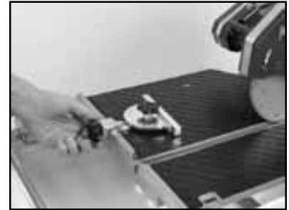
(C) Position the 90° Protractor and tighten the retaining thumbscrew.
