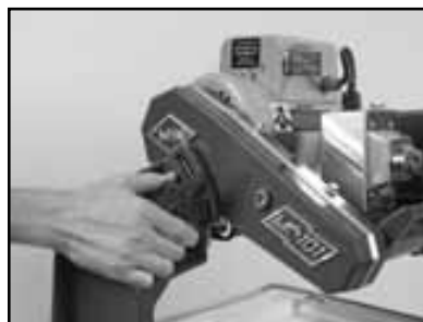
(A) Loosen Cutting Head Adjusting Knob.
