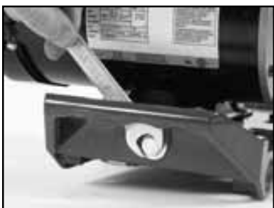
(M) Tighten the Motor Adjustment Strap to remove slack.
