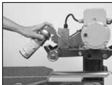
(H) Lubricate the Blade Guard Pivot Shaft.
