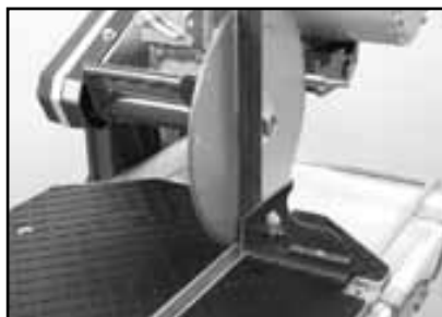
(B) Position Square on Movable Cutting Table against the Diamond Blade.
