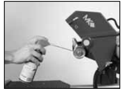
(C) Lubricate the Arbor Shaft.
