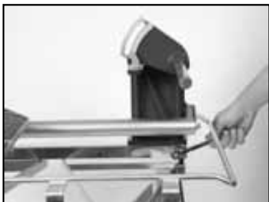
(G) Install and tighten the Post Support Plate and retaining bolts.
