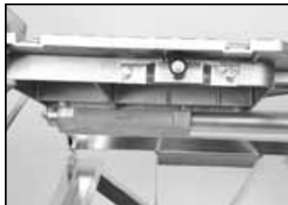
(E) Move Wheel Assembly up or down to Square the Movable Cutting Table.
