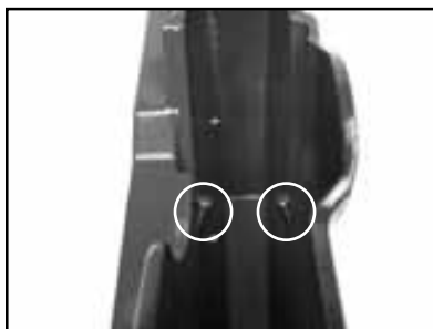
(D) Verify proper cooling flow on both sides of the blade (See Maintenance Section to increase/decrease flow).
