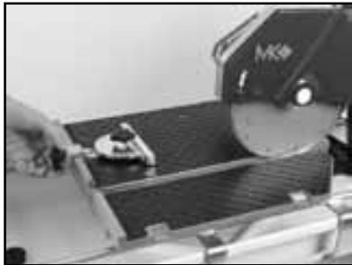
(A) Place the 90° Protractor on the Ruler/Stop.
