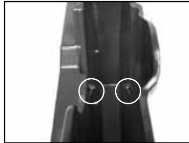
(E) Verify proper cooling flow on both sides of the blade (See Maintenance Section to increase/decrease flow).
