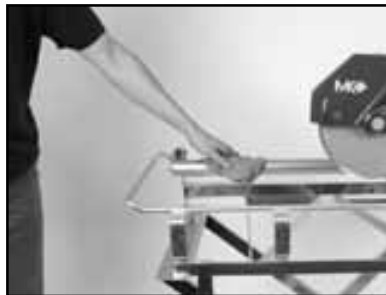
(E) Clean the Movable Cutting Table Guide Bar.
