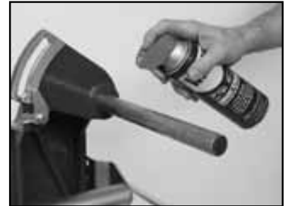
(L) Lubricate the Cutting Head Pivot Shaft.
