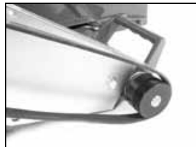
(L) Verify the V-belt is seated in the grooves of both pulleys.
