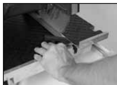
(C) Move the Cutting Table back and forth to re-verify Blade is even across all points of Square.
