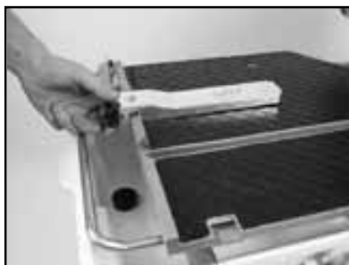
(A) Remove the Adjustable Cutting Guide.
