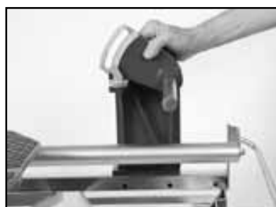
(F) Relocate the Post to the rear Post retaining holes.
