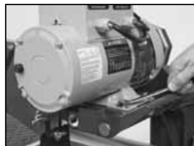
(G) Loosen the motor mounting bolts, if re-tensioning only go to step M.
