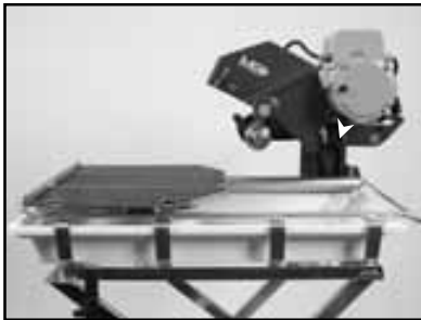
(A) Position Movable Cutting Table to the front of the saw and raise the Blade Guard by loosening the wingnut.
