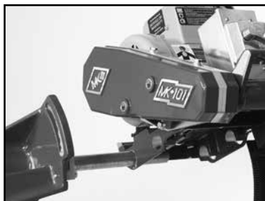
(B) Remove the Cutting Head (See Adjusting the Cutting Head).
