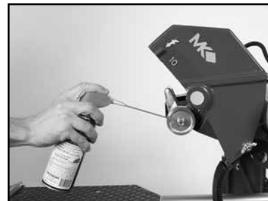
(C) Lubricate the Arbor Shaft.
