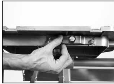
(E) Move Wheel Assembly up or down to Square the Movable Cutting Table.
