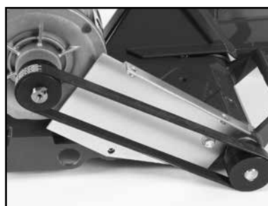
(E) Inspect the belt for cracks, fraying, separation and wear. Go to step I if replacement required.
