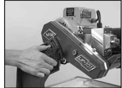
(C) Tighten the Adjusting Knob.
