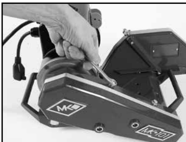
(Q) Install the Belt Guard. Tighten all three bolts
