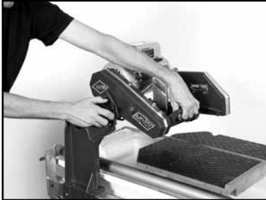
(A) Loosen Cutting Head Adjusting Knob.
