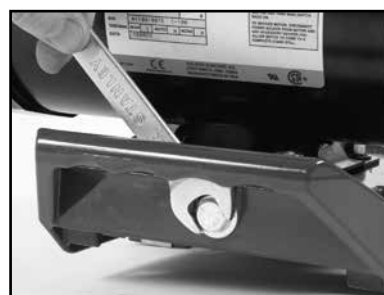
(H) Loosen the Motor Adjustment Strap.
