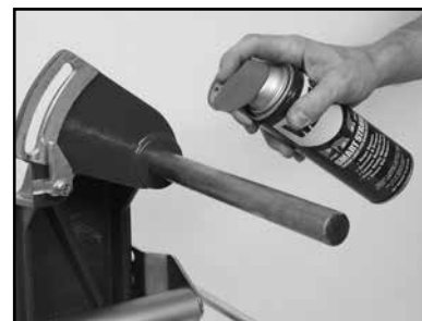
(L) Lubricate the Cutting Head Pivot Shaft.
