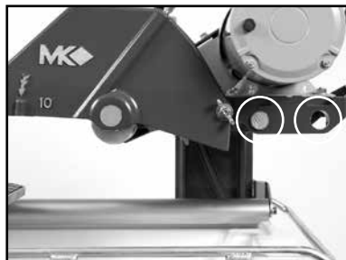
For maximum cutting length, the Cutting Head should be in the front pivot hole and the Post should be in the rear post retaining hole.
