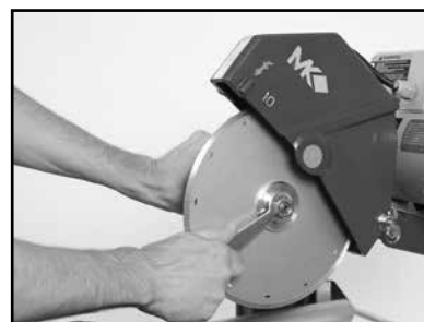
(F) Install Retaining Nut and Outer Flange, depress and hold the Shaft Lock pushbutton and tighten Retaining Nut.
