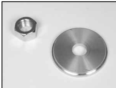
(B) Lubricate the Outer Flange and Retaining-nut.
