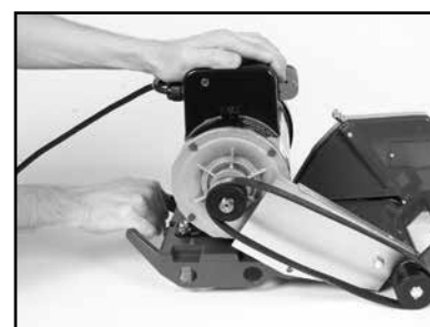
(I) Push the motor toward the front of the Cutting Head to loosen the belt.
