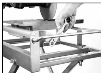
(B) Tighten Guide Bar Retaining Bolts.
