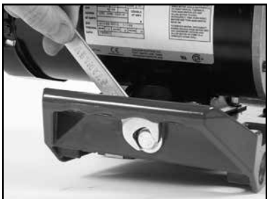
(M) Tighten the Motor Adjustment Strap to remove slack.
