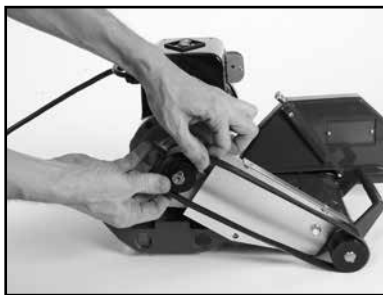
(K) Install the new belt.
