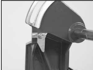
(B) Remove the Cutting Head Stop Bolt. Rotate Cutting Head Stop to down position and re-tighten Cutting Head Stop Bolt.
