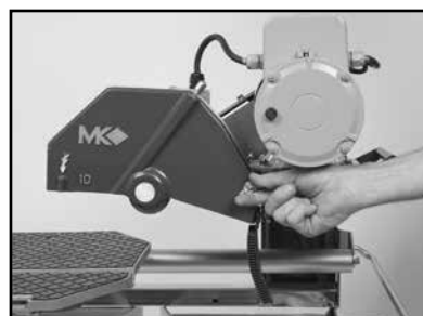
(G) Remove the Blade Guard.
