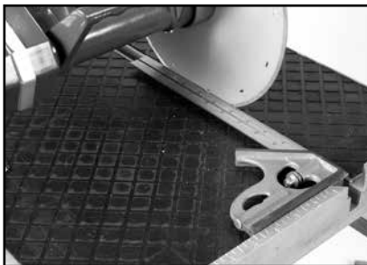
(D) Position Square flat on Movable Cutting Table against Ruler/Stop. Position front of Square against Blade.
