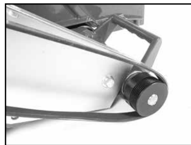
(L) Verify the V-belt is seated in the grooves of both pulleys.
