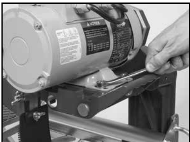
(P) Tighten the motor mounting bolts.
