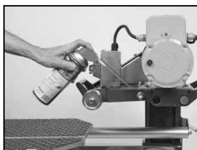
(H) Lubricate the Blade Guard Pivot Shaft.
