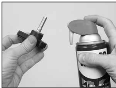
(J) Lubricate the Cutting Head Adjustment Knob.
