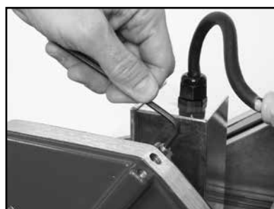
(F) Remove the Cooling Channel cover screws. Go to step G.
