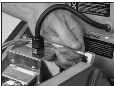
(B) Remove the Cooling Transfer Tube from the Blade Guard inlet. Go to Step C.
