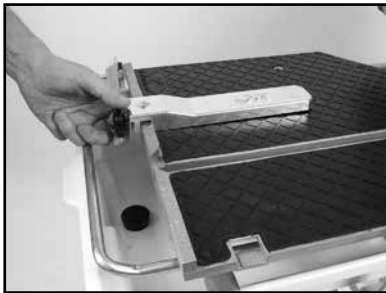
(A) Remove the Adjustable Cutting Guide.
