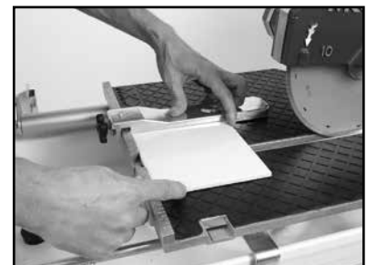
(C) Place the tile against the Ruler/Stop and Cutting Guide. Turn the motor ON.
