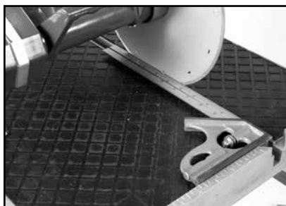
(A) Move the Cutting Table back and forth to verify Blade is even across all points of Square.
