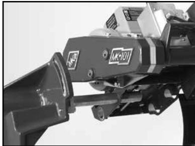
(A) Align Cutting Head front Pivot Hole to the Post Shaft and slide onto shaft.
