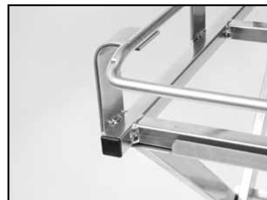
(C) Ensure the back of the saw frame is positioned properly
