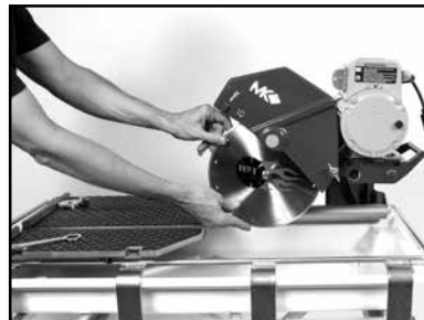
(E) Install Diamond Blade onto Blade Shaft.
