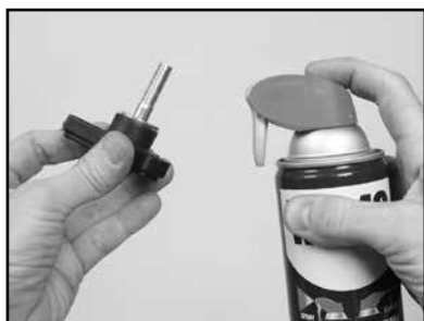
(J) Lubricate the Cutting Head Adjustment Knob.
