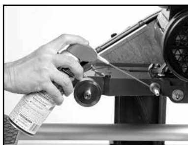
(H) Lubricate the Blade Guard Pivot Shaft.
