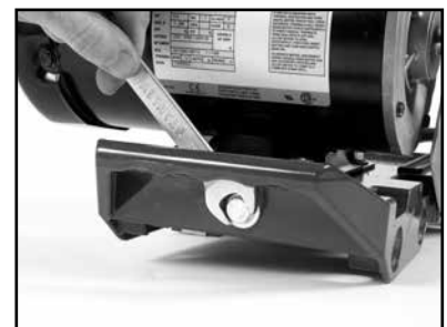
(I) Loosen the Motor Adjustment Strap
