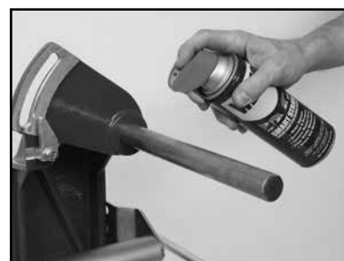
(L) Lubricate the Cutting Head Pivot Shaft.
