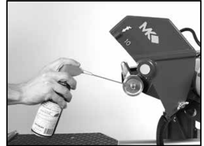
(C) Lubricate the Arbor Shaft.
