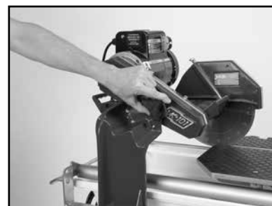
(C) Tighten the Adjusting Knob.
