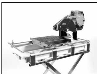
(E) Reinstall the Water Basin
