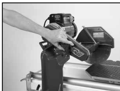
(A) Loosen Cutting Head Adjusting Knob.
