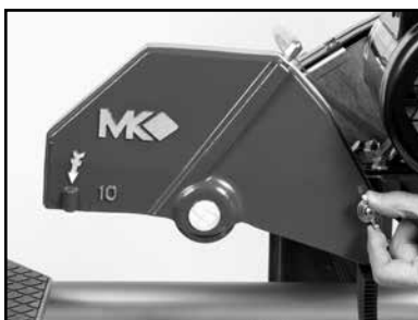
(G) Remove the Blade Guard.
