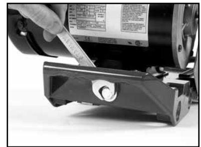
(I) Loosen the Motor Adjustment Strap
