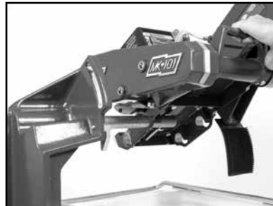
(E) Install the Cutting Head onto the front pivot hole.
