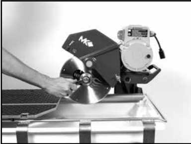
(A) Remove the Diamond Blade.
