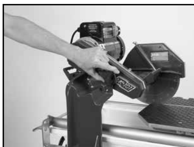
(A) Loosen Cutting Head Adjusting Knob.
