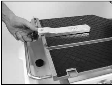
(A) Remove the Adjustable Cutting Guide.
