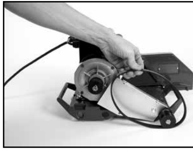
(K) Remove the Micro-V Belt
