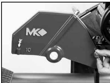
(G) Remove the Blade Guard.
