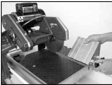
(A) Position the 45° Bullnose Miter Guide and tighten the retaining thumbscrew.
