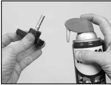
(J) Lubricate the Cutting Head Adjustment Knob.
