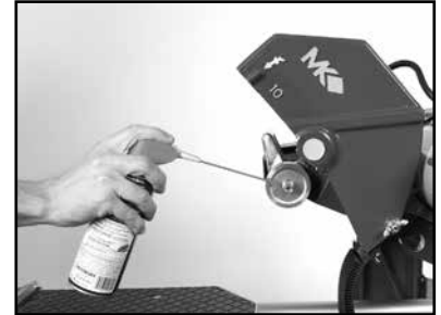
(C) Lubricate the Arbor Shaft.
