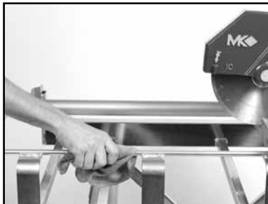
(E) Clean the Movable Cutting Table Roller Wheel Frame Support.
