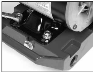
(H) Loosen the two back motor mounting bolts
