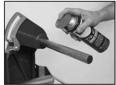
(L) Lubricate the Cutting Head Pivot Shaft.
