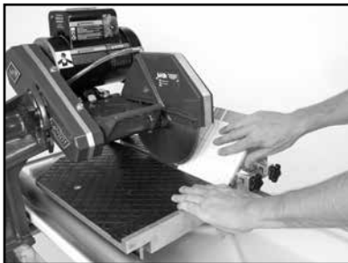
(D) Perform the cut. Turn the motor OFF when work is complete.
