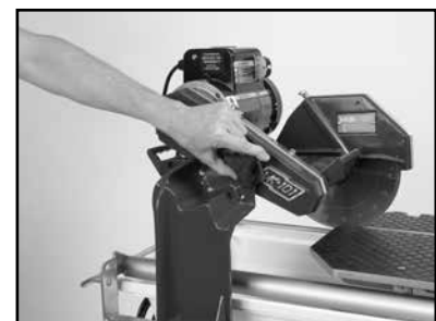
(C) Tighten the Adjusting Knob.
