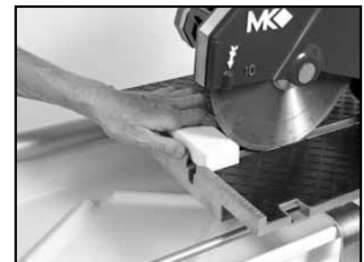
(C) Position the Dressing Stick. Cut 2 or 3 strips from the dressing stick to dress the Blade.
