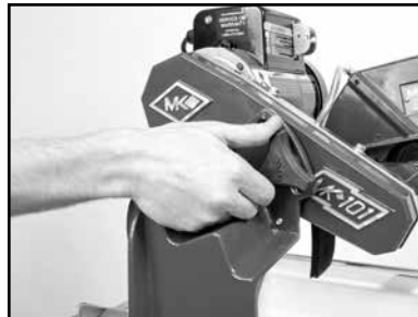
(B) Remove the Blade. Remove Adjusting Knob.
