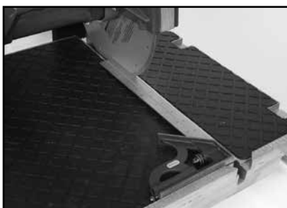
(D) Position Square flat on Movable Cutting Table against Ruler/Stop. Position front of Square against Blade.
