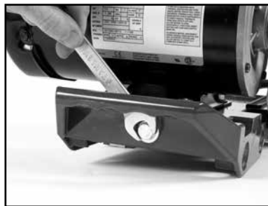
(N) Tighten the Motor Adjustment Strap to remove slack
