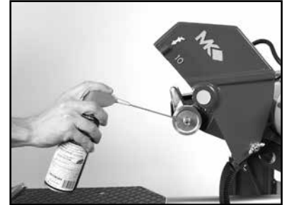
(C) Lubricate the Arbor Shaft.
