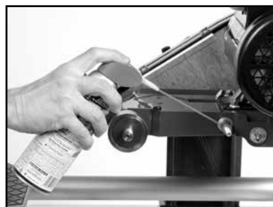
(H) Lubricate the Blade Guard Pivot Shaft.
