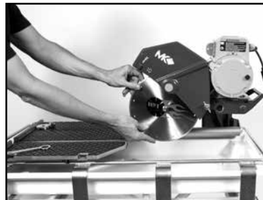
(E) Install Diamond Blade onto Blade Shaft.
