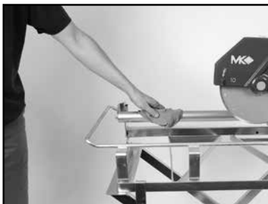
(A) Check the Guide Bar and Frame for cleanliness – clean if dirty.
