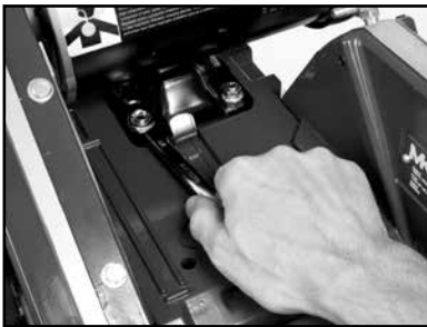
(P) Tighten the four motor mounting bolts
