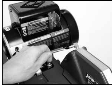
(B) Remove the Cooling Transfer Tube from the Blade Guard inlet. Go to Step C.
