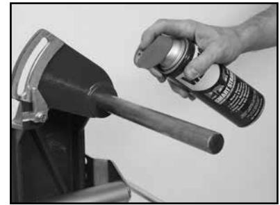
(L) Lubricate the Cutting Head Pivot Shaft.
