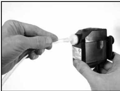
(D) Remove the Cooling Transfer Tube and check for flow. If flow exists, refer to water pump manual.
