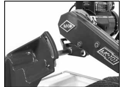
(C) Remove the Cutting Head from the rear pivot hole.
