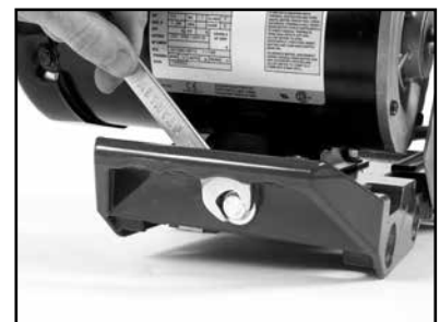
(I) Loosen the Motor Adjustment Strap
