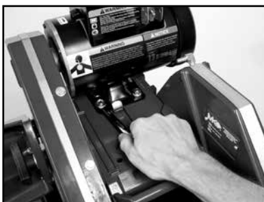
(G) Loosen the two front motor mounting bolts. If re-tensioning only, go to step N
