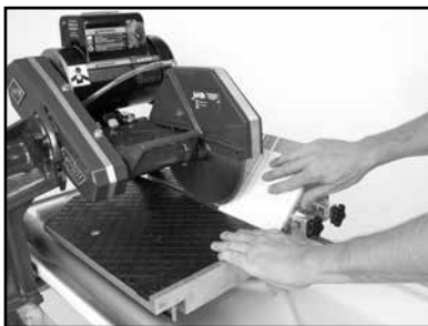
(D) Perform the cut. Turn the motor OFF when work is complete.
