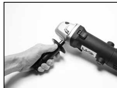
(C) Or install the straight handle by rotating clockwise to tighten. It may be installed on left or right side.
