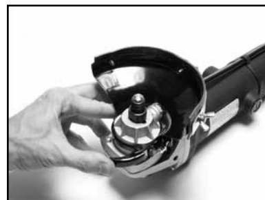
(C) Secure Shroud by closing lever clamp.
