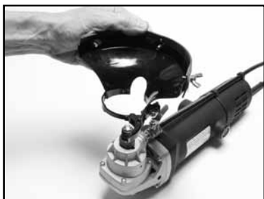
(A) Place Shroud on polisher with the lever clamp open.
