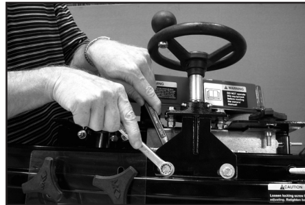
Fig. 33 Major vertical (Pre-set for normal operation adjustments)
