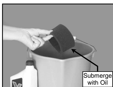
(E) Dip Foam Filter in clean engine oil – Squeeze out excess oil
