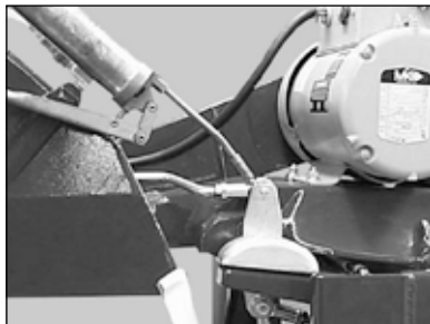
(G) Apply grease to the nine (9) Zerk Fittings of the MK-5000 (See Unit Lubrication page 32).
