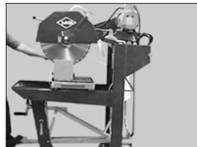
(F) Lower cutting head an ad- ditional 1/4" to 1/2" with Foot Pedal for "Pull" Stroke.
