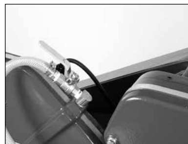
(C) Open the Cooling Flow Control Valve and adjust flow. Verify proper cooling flow on both sides of the blade.
