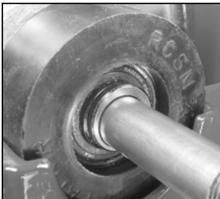
Fig 35 - Bearing correctly installed
