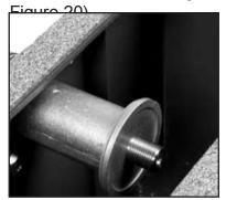
Figure 19: Blade Arbor and Inner Flange
