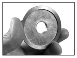
Figure 22: Convex (recessed) Side of the Blade Flange
