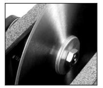
Figure 20: Blade Arbor Blade, Outer Flange, and Jam Nut
