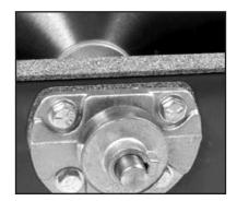
Figure 16: Arbor Housing Mounting Bolts
