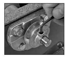
Figure 17: Pulley Setscrew
