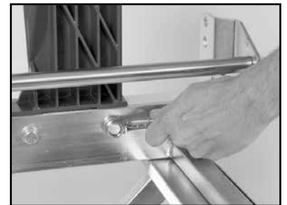
(C) Loosen the Retaining Bolts.
