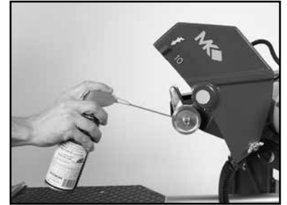
(C) Lubricate the Inner Flange.
