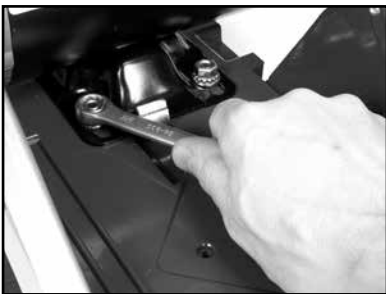
(P) Tighten the four motor mounting bolts.
