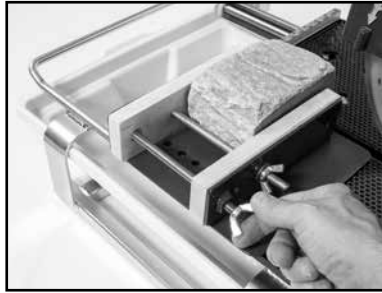
(B) Tighten wingnut farthest from material.
