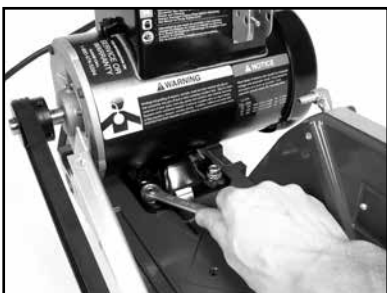
(G) Loosen the two front motor mounting bolts. If re-tensioning only, go to step N.
