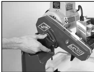
(E) Install the Adjusting Knob.
