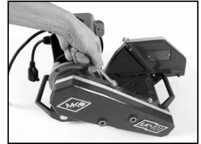
(C) Remove the two top Belt Guard Bolts.
