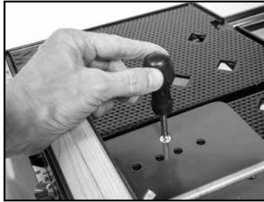
(B) Place screws through top of table.
