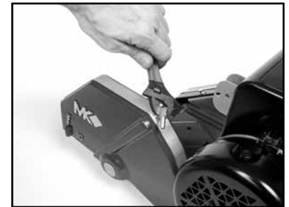
(F) Remove the Blade Guard In- take Fitting and check.
