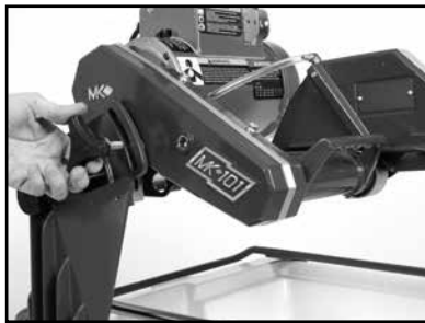
(A) Ensure the ON/OFF Switch is in the OFF position. Remove the blade and then Adjusting Knob.
