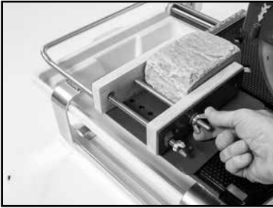
(A) Place material in vise. Tighten wingnut closest to material first.
