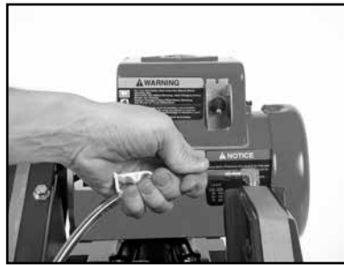
(B) Remove the Cooling Transfer Tube from the Blade Guard inlet.
