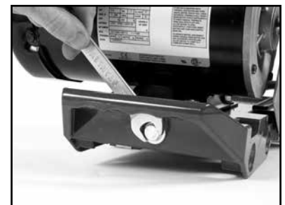
(I) Loosen the Motor Adjustment Strap.
