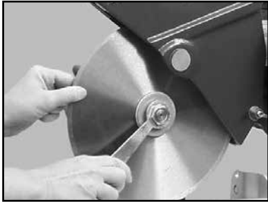
(A) Remove the Diamond Blade.
