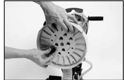
Insert the four bolts and tighten.
