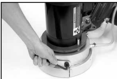
Insert Allen wrench and unscrew bolt. Repeat on other side of shroud.
