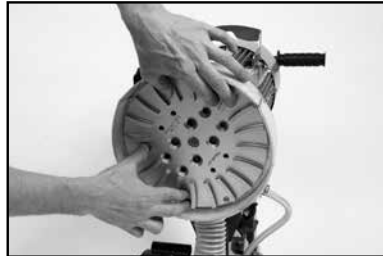
Place Grinding Disc on mounting plate, aligning bolt holes.
