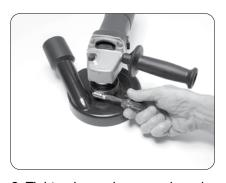
**3.** Tighten hose clamp so shroud is firmly attached to grinder.
