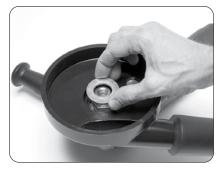
If necessary place large washer(s) on cup adapter nut, so cup wheel extends 1/16" to 1/8" beyond shroud.
