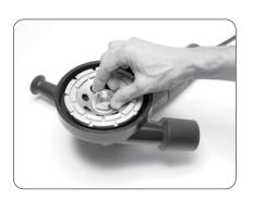
Screw hex nut onto cup nut assembly.
