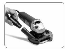
Attach hose adapter. Shroud is now ready to be attached to vacuum.
