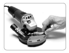
**8.** Close quick release latch so shroud is firmly attached to grinder. Ensure cup wheel does not contact shroud and extends 1/16" - 1/8" below shroud.
