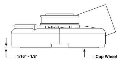
**NOTE:** Use washer(s) to achieve proper distance if needed. As cup wheel is worn use additional washer to achieve distance needed.
