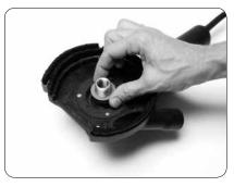
5. If necessary place large washer(s) on cup adapter nut, so cup wheel extends 1/16" to 1/8" beyond shroud.
