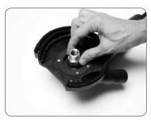
**4.** Screw cup adapter nut on grinder arbor shaft.
