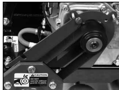
(C) Inspect the belt for excessive wear, cracks and cuts – if worn, proceed to Step E.
