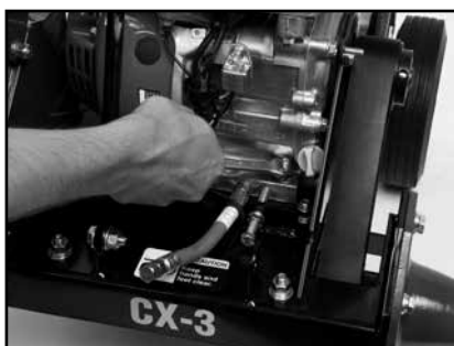
(E) Locate the four upper Engine Mounting Nuts on both ends of the CX-3® motor and loosen.
