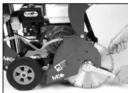
(F) Tighten Blade Retaining Bolt while holding the Blade Shaft steady.
