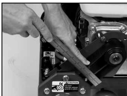
(D) Check belt for proper tension if ten- sion is correct, go to Step P (Proper tension is approximately 1/8-inch deflection of the belt).
