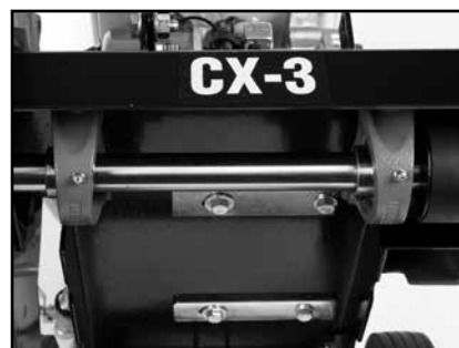
(F) Locate the four lower Engine Mounting Bolts on both ends of the CX-3® motor and loosen.
