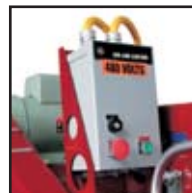
NEMA 12 waterproof enclosure with heavy-duty starter. Safety Switch prevents accidental restart if electrical current is disrupted
