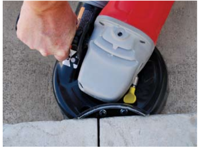
The IXL hinged shroud is designed for grinding against walls and edges.
