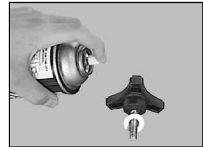
(L) Lubricate the Cutting Head Adjustment Knob
