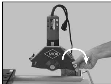
(J) Tighten the Blade Guard Retaining, Wing nut
