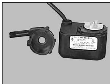
(H) Remove the Pump Casing and check for restriction; check Impeller damage
