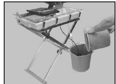
(C) Fill the external container until water completely covers the Water Pump suction
