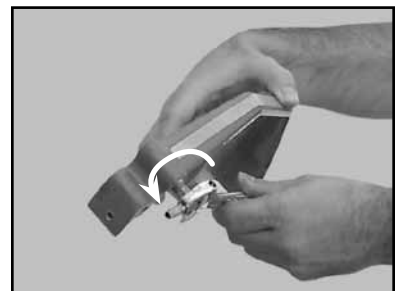
(I) Remove the Blade Guard Intake Fitting
