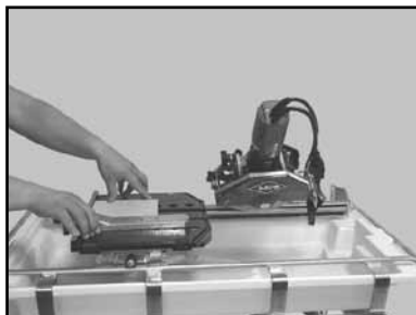
(G) Place the tile against the Ruler/Stop and Cutting Guide
