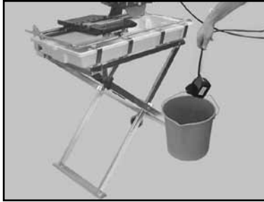
(B) Place the Water Pump in an external container
