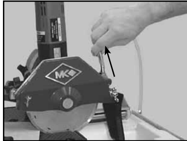
(B) Remove the Cooling Transfer Tube from the Blade Guard inlet
