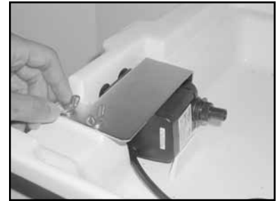
(C) Secure Clamp with 1/4-20 wing screws and nuts.
