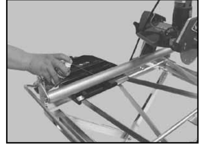
(C) Lubricate the Guide Bar
