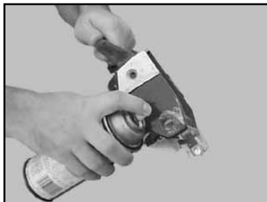
(J) Lubricate the Cutting Head Pivot Holes
