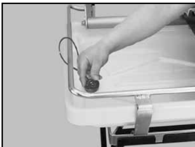
(A) Remove the Drain plug
