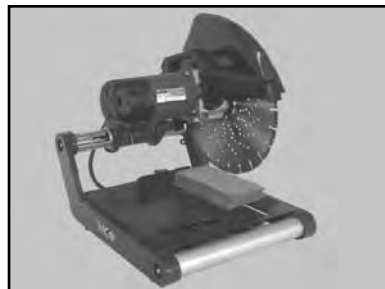
Position work against back stop as shown and perform the cut
