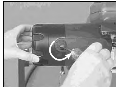
(E) Change the second Motor Brush by repeating steps (A) to (D)
