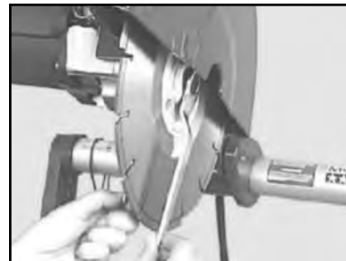
(E) Install the Retaining Nut and Outer Flange and then tighten using the Blade and Shaft Wrenches
