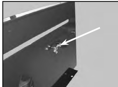
Loose wingnut located underneath the table
