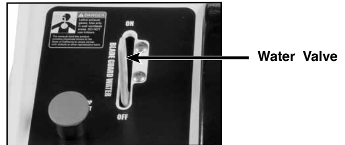
Fig. 17 Partially open Water Valve
