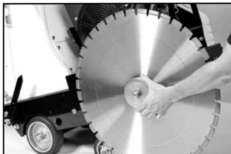
Fig. 11 Slide Outer Flange in place
