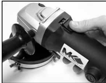
(E) Place the ON/OFF Switch in the OFF position.
