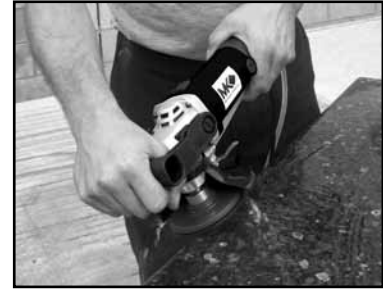
(C) Using the coarse grit disc, re- move all rough scratches and cut marks.
