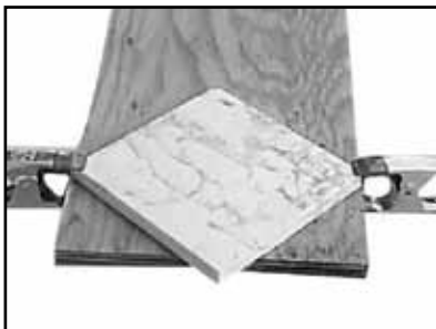
(A) If necessary, clamp the material to be polished to a work surface.
