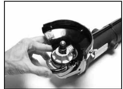
(C) Secure Shroud by closing lever clamp.
