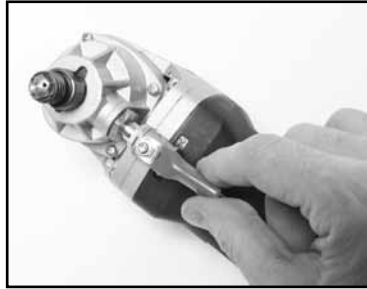
(B) Adjust water flow (excessive water flow can result in internal electrical problems).
