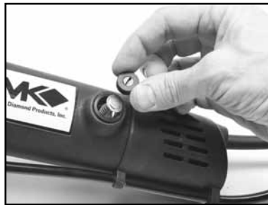
(E) Using a flat blade screwdriver install the Motor Brush Housing cover.
