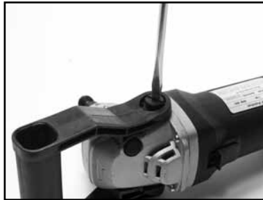
(B) Tighten bolts on both sides.
