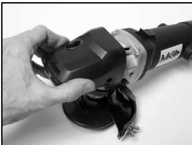
(A) Slide on Motor Cover and secure with bolts.
