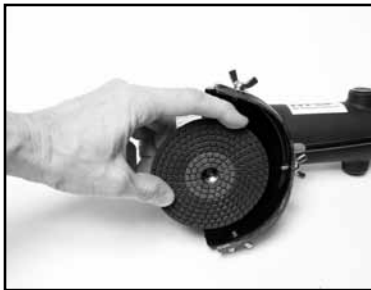
(A) Align the Velcro Polishing Disc to the Backer Pad. Press disc evenly and firmly onto the Backer Pad.
