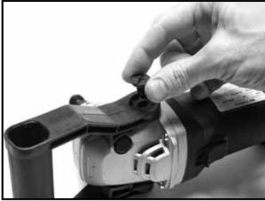
(A) Place D-Handle on polisher and insert bolt.
