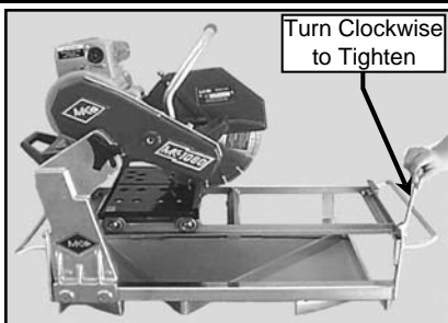
(B) Tighten front and rear Adjustable Frame Adjusting Bolts
