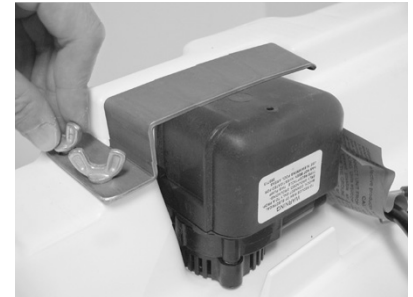
(C) Secure Clamp with ¼-20 wingscrews and nuts.
