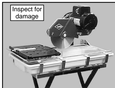
(E) Inspect the MK-100 TRACKER for damage – ensure the cord is free of cracks or cuts
