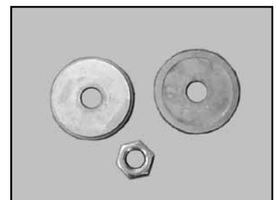
(C) Clean and Lubricate the Inner and Outer Flanges and the Retaining Nut
