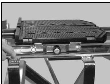
(M) Verify the Cutting Table Roller Wheel Assembly is tight
