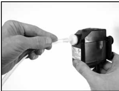
(D) Remove the Cooling Transfer Tube and check for flow. If flow does not exist, refer to water pump manual.
