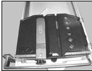
(E) Position the Adjustable Cutting Guide to desired cut length indicated inside the diamond
