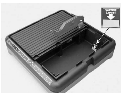
2: Water Level Warning
