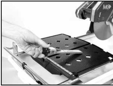
(A) Loosen the Adjustable Cutting Guide retaining thumbscrew
