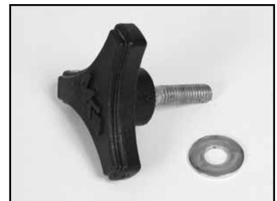
(I) Lubricate the threads on the Cutting Head Adjustment Tri-Knob
