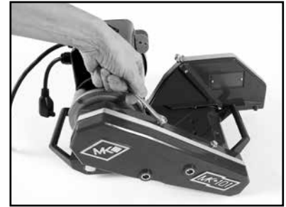
(C) Remove the two top Belt Guard Bolts
