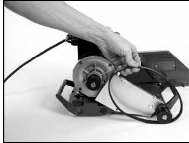
(K) Remove the Micro-V Belt
