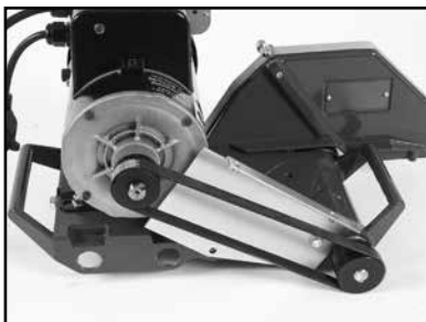
(A) Check and adjust V-belt tension following first 48 hours of operation (See V-belt Inspection).
