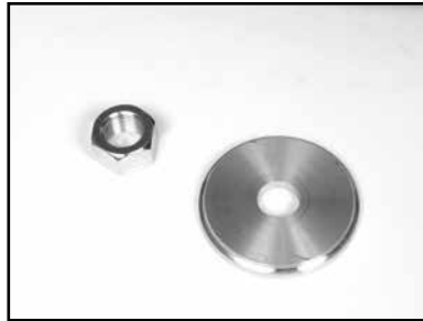
(B) Clean and lubricate the Outer Flange and Retaining-nut
