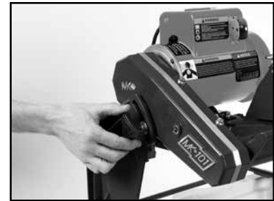
(C) Ensure the Cutting Head Tri- Knob is tight
