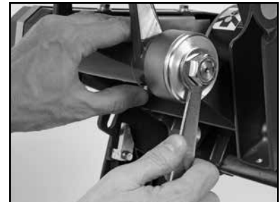
(C) Depress and hold the Shaft Lock button and remove Retaining Nut and Outer Flange using the Blade Wrench
