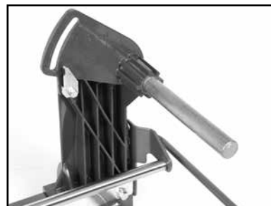
(K) Lubricate the Cutting Head Pivot Shaft
