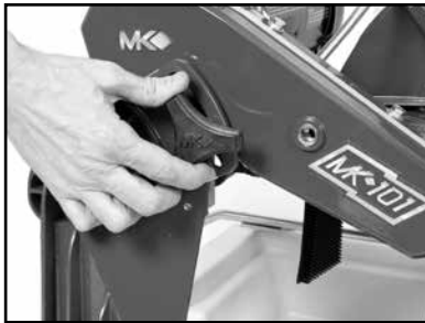
(A) Loosen Cutting Head Tri- Knob and move cutting head down
