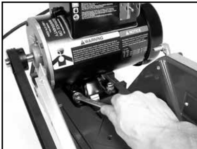
(P) Tighten the four motor mounting bolts
