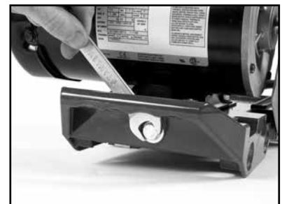
(I) Loosen the Motor Adjustment Strap
