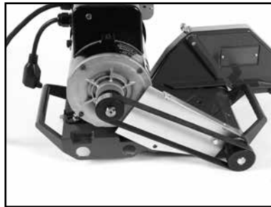
(E) Inspect the Micro-V Belt for cracks, fraying, separation and wear. Go to step H if replace- ment is required
