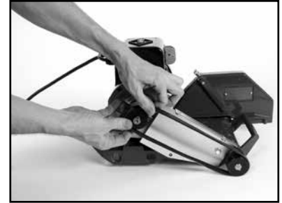
(L) Install the new Micro-V Belt (MK Diamond Part No. 158194)
