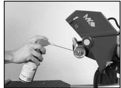
(C) Lubricate the Arbor Shaft
