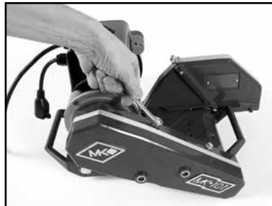
(Q) Install the Belt Guard
