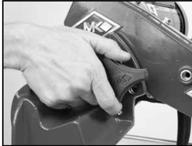
(B) Install the Cutting Head onto the Post Pivot Shaft and install the Cut- ting Head Tri-Knob and washer.
