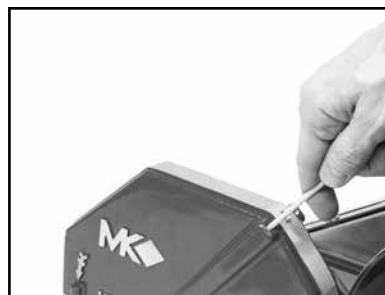
(H) Rod Cooling Channels and recheck flow
