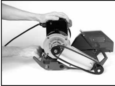
(J) Push the motor toward the front of the Cutting Head to loosen the Micro-V Belt
