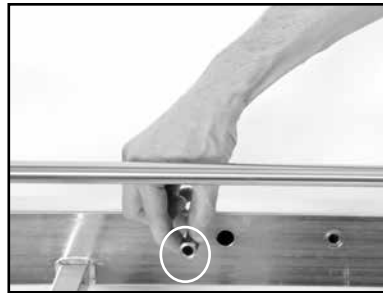
(E) Move Standoff and bolt to rear post retaining hole
