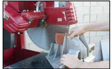
Adjust jig to desired width.
