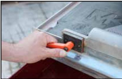
Lock jig in place with orange lever.
