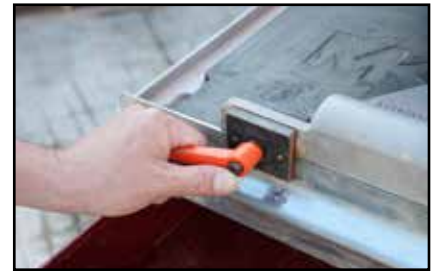
Lock jig in place with orange lever.
