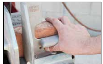
Place right-hand on jig. Start cutting.
