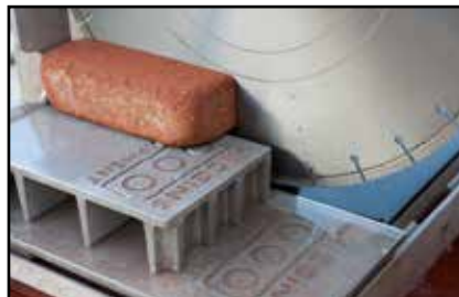
Pull table back through brick and flip brick.
