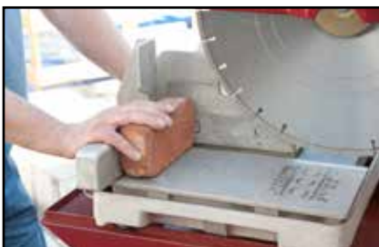
Place brick on table and turn on saw.
