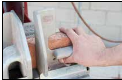
Adjust the height of the cutting head to the desired depth and lock down. Adjust jig to desired width.
