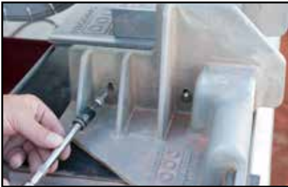
Attach riser plate to jig by tightening the two screws.
