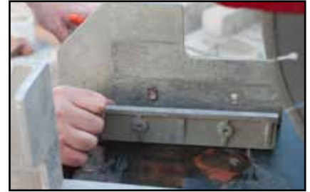
Place riser plate to inside of jig.
