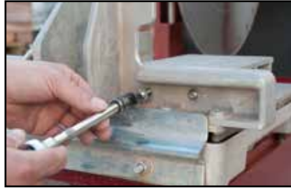
Attach riser to jig by tightening the two bolts.
