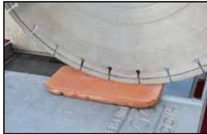
Adjust the height of the cutting head to the desired depth and lock down.
