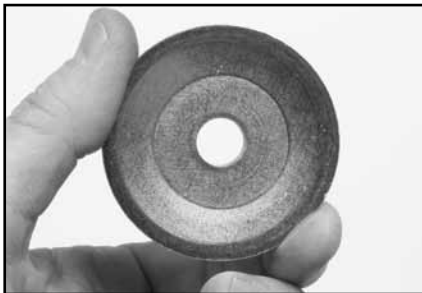
Figure 20: Convex (recessed) Side of the Blade Flange
