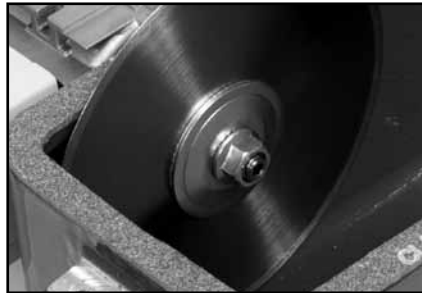
Figure 18: Blade Arbor Blade, Outer Flange, and Jam Nut
