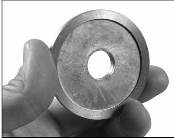
Fig 35. Convex or recessed side of blade flange
