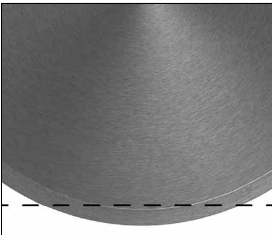
Fig 4. Coolant level should cover the bottom 1/4" of the blade
