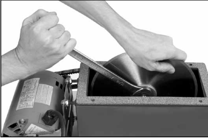
Fig 34. Hold the blade with one hand use a 15/16" wrench to turn the jam nut. Do not over tighten
