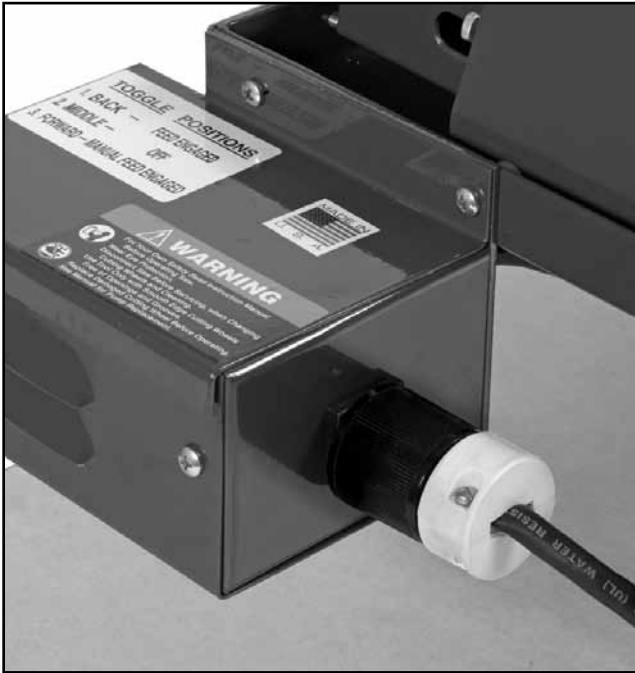
Fig 9. Motor cord attached to the power feed box receptacle
