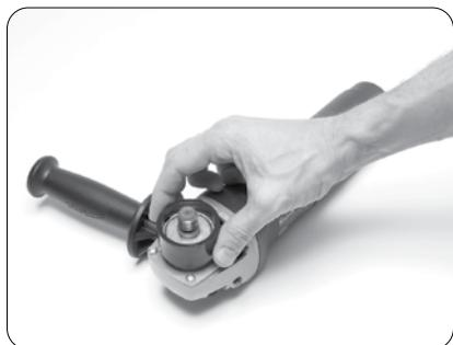
1. If grinder has a small throat, use collar so shroud fits tightly.
