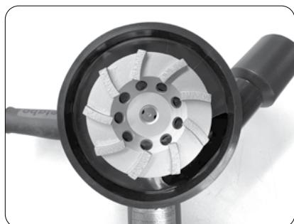
4. Attach cup wheel. Ensure cup wheel does not contact shroud.
