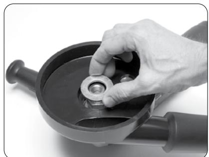
3. If necessary place large washer(s) on cup adapter nut, so cup wheel extends 1/16" to 1/8" beyond shroud.
