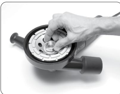
5. Screw hex nut onto cup nut assembly.
