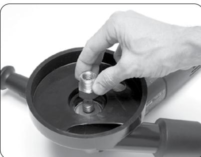
2. Screw cup adapter nut on grinder arbor shaft.
