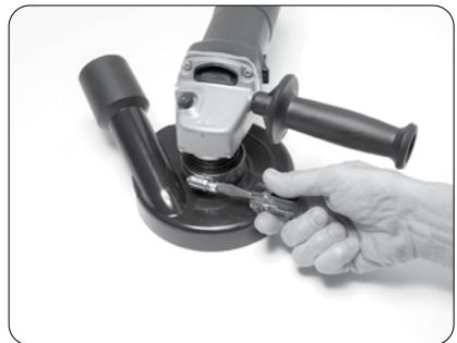
3. Tighten hose clamp so shroud is firmly attached to grinder.
