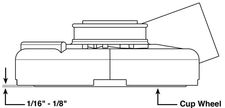
**NOTE:** Use washer(s) to achieve proper distance if needed. As cup wheel is worn use additional washer to achieve distance needed.
