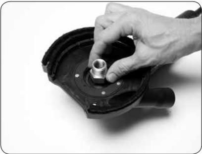
4. Screw cup adapter nut on grinder arbor shaft.
