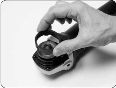
1. If grinder has a small throat, use bushing so shroud fits tightly.
