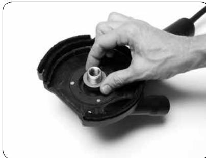
5. If necessary place large washer(s) on cup adapter nut, so cup wheel extends 1/16" to 1/8" beyond shroud.
