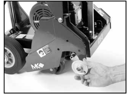
(C) Remove the Inner Blade Flange.
