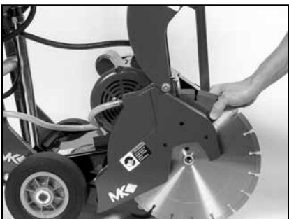
(A) Remove the Blade (See Blade Removal section).
