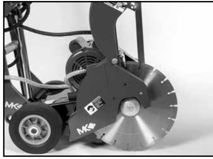
(B) Push Lock Button. Open the Blade Guard Cover.
