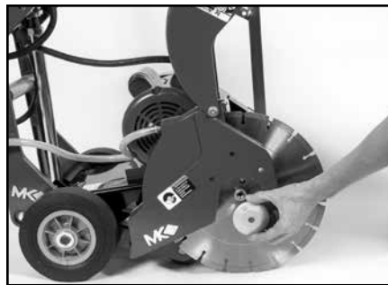
(E) Install the new Blade, Retaining Bolt and Outer Flange.
