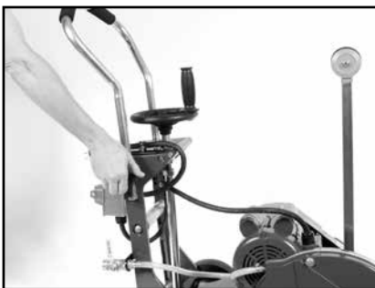
(A) Loosen the Tri-Knobs on both sides of the Handlebar.
