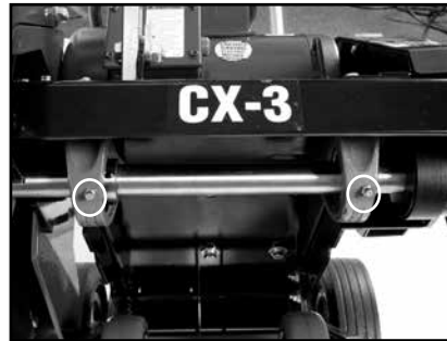
(B) Lubricate the Blade Shaft Bear- ings (Monthly).
