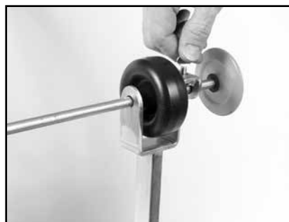
(N) Switch orange Pointer wheel to align with blade.
