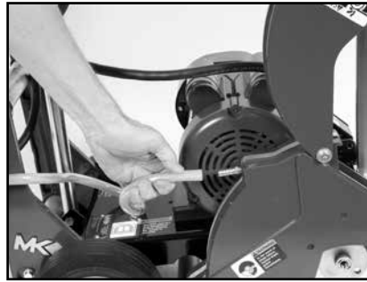
(B) Remove the Cooling Transfer Hose from the Blade Guard.
