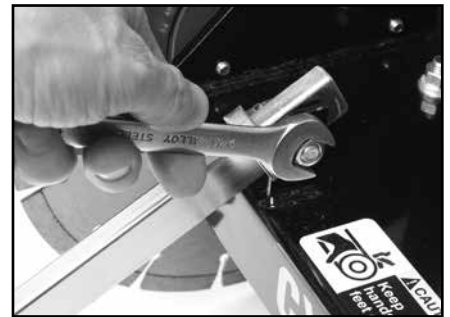
(C) Thread locking nut on to bolt and tighten.
