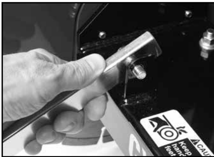
(A) Insert bolt on Pointer into mounting flange next to Blade Guard.
