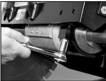
Loosen 4 bolts on the two retaining caps so gearbox can rotate.
