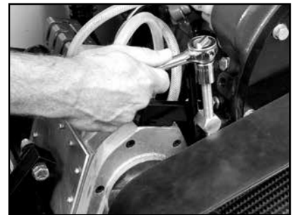
Apply tension to belt by turning tension screw clockwise, increasing tension.
