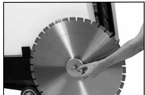
Slide Outer Flange and Arbor bolt in place
