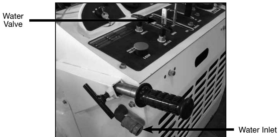
Water Hook Up
