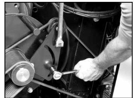
To Tension Belt: Loosen locknut on tension arm. Apply tension with 1/2" drive breaker bar.
