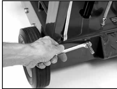
(K) Tighten the Engine Tension Arm Nut.
