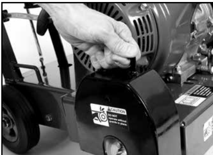
(G) Install the Blade Shaft Cover and tighten bolts.
