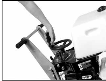
(B) Lower the MK-1318 to its lowest position.
