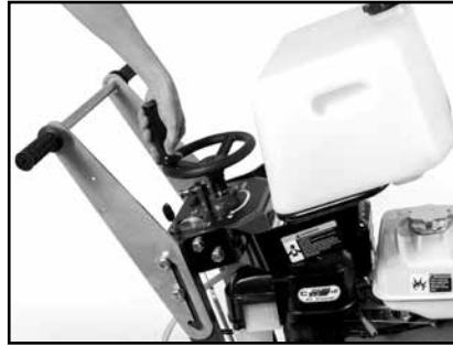
(B) Turn Crank Wheel until Blade touches the ground.
