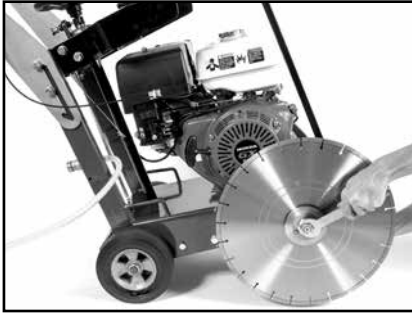
(A) Remove the Blade Guard and Diamond Blade. See Blade Removal section.
