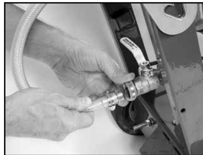
(B) Attach the water hose to the Cooling Inlet, if wet cutting.
