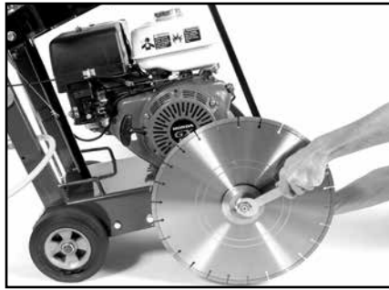
(H) Tighten Blade Shaft Nut holding the Blade Shaft steady.
