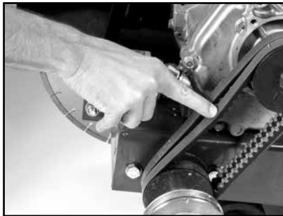
(D) Check belt for proper tension if tension is correct, go to Step P (Proper tension is approximately 1/8-inch deflection of the belt).
