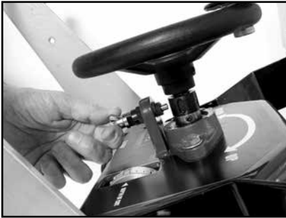
(A) Unlock Crank Wheel.
