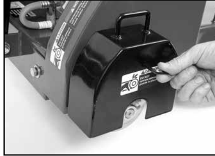
(B) Locate the Blade Shaft Cover locking bolt hole.
