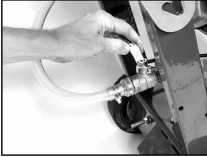
(E) Lubricate the Cooling Supply Valve.
