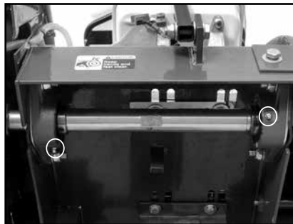
(B) Lubricate the Blade Shaft Bearings (Monthly).
