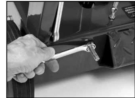
(F) Loosen the Engine Tension Arm adjusting nut. Push the Engine forward to loosen the belt.
