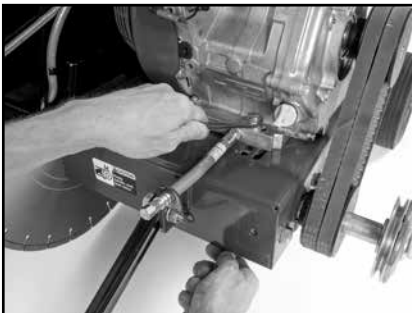
(M) Tighten the Engine Mounting Bolts.
