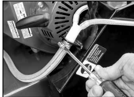
(E) Remove water hose from blade guard.
