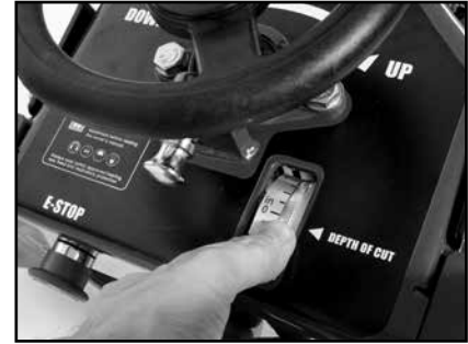
(C) Set depth indicator to zero.
