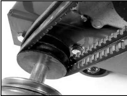
(J) Verify the belts are seated in all grooves of the Blade Shaft Pulleys.
