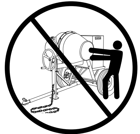
Fig 3. Filling Mixing Drum
